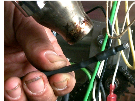
Fig: 10 Apply heat to secure the shrink wrap in place.
