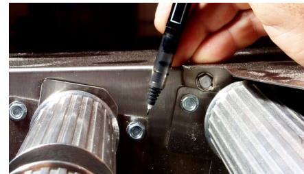
Fig: 11 This screw on the controller side of the front upper roller is removed to accommodate the placement of a crumb catcher.
