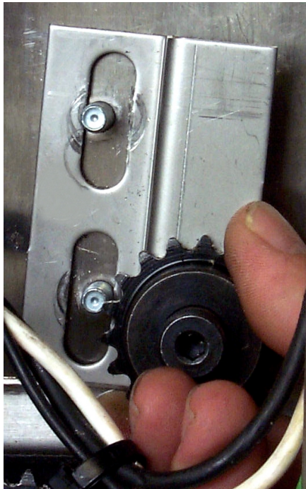
Fig 4: Cock the idler assembly, as shown to ensure proper tension on the chain and tighten nuts. (Shown with chain off to reveal position of studs.)
